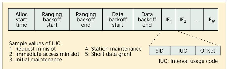
FIGURE 6. DOCSIS bandwidth management PDU format.
