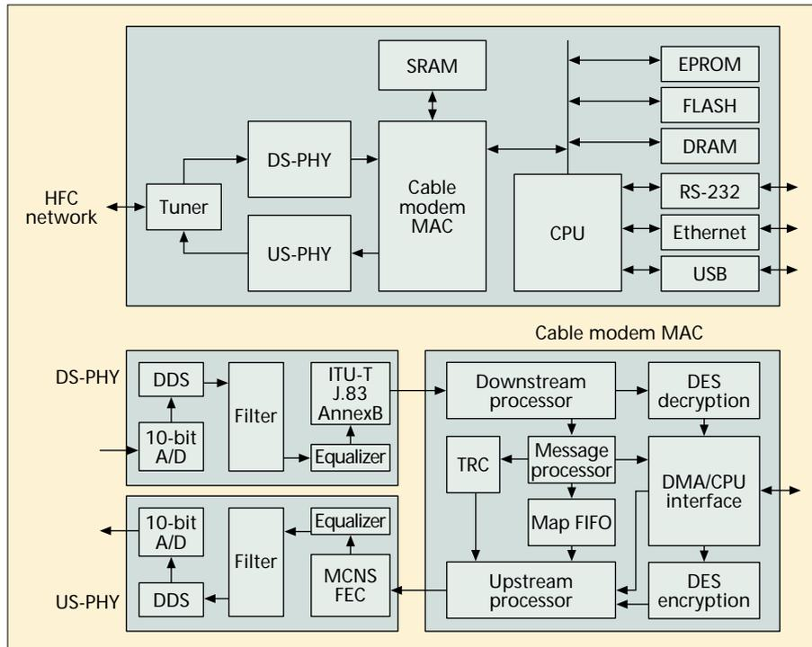
■ FIGURE 8. The hardware architecture of the cable modem.
