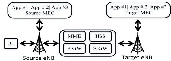
Fig. 1. MECs deployed in 4G LTE Network
