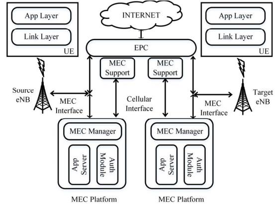
Fig. 2. Proposed MEC integrated cellular system architecture
