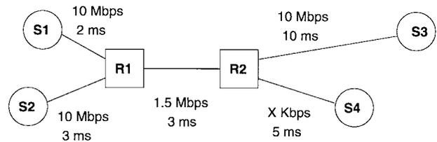
Fig. 1. Simulation network.
