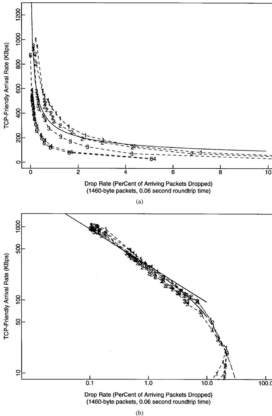
Fig. 10. TCP-friendly bandwidth for a 60-ms round-trip time and 1460-byte packets.
