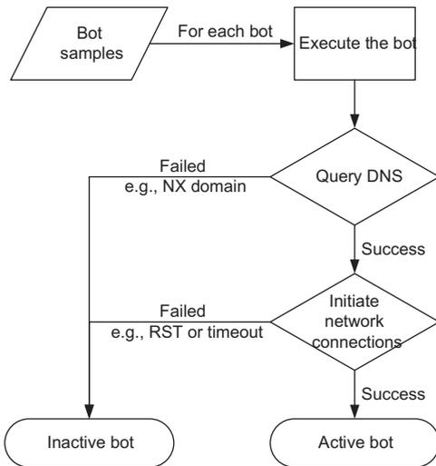
Fig. 4. The procedure of a bot's execution.
