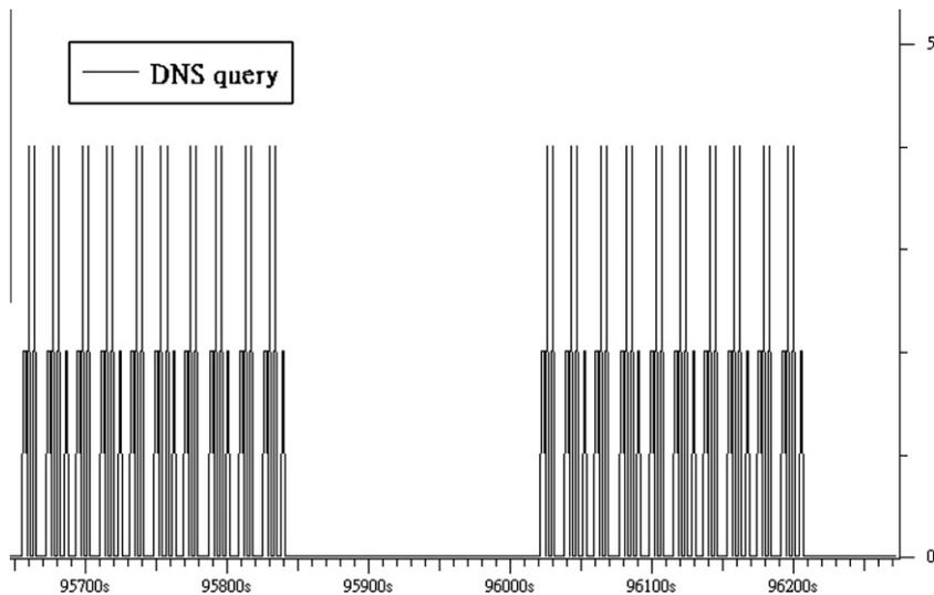
**Fig. 6.** The distribution of botnet DNS query packets generated by the “Backdoor.Win32.SmallBot.c” bot: interleaved intervals pattern (x-axis: interval in seconds; y-axis: number of DNS query packets).
