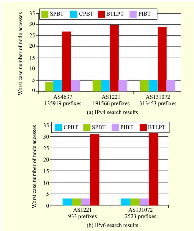
Fig. 10. Worst case node accesses results of search procedures for B-tree schemes (IPv4 and IPv6 databases).
