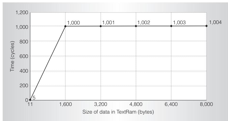
Figure 2. Scanning time for various data lengths.
