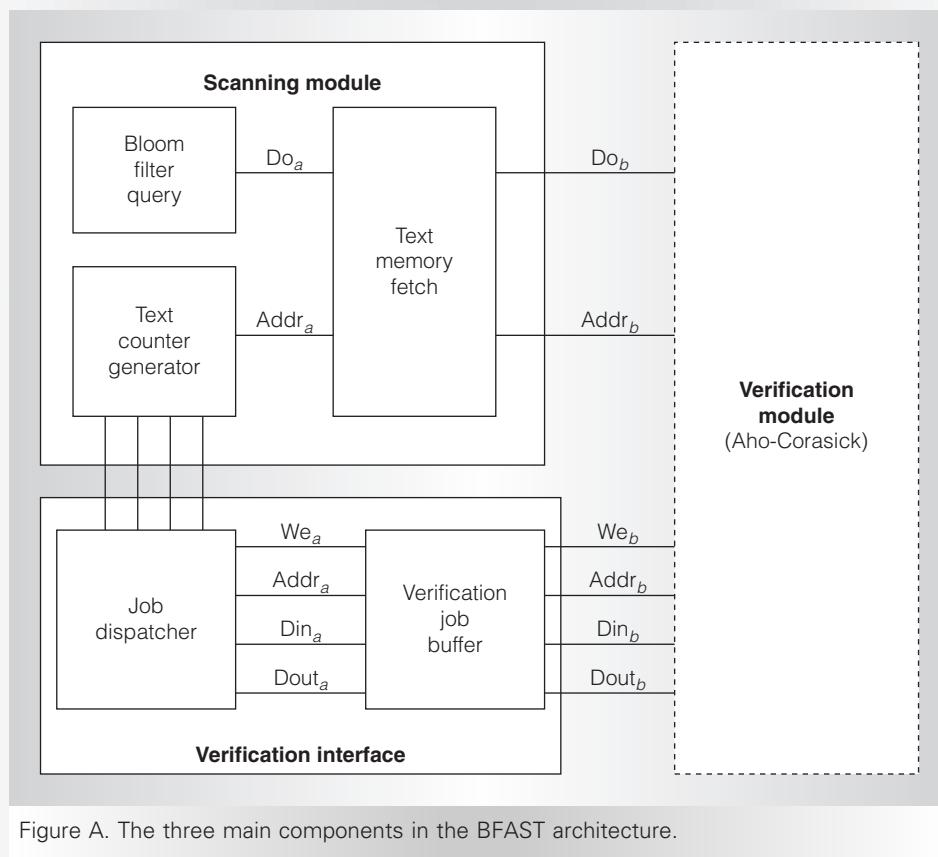
Figure A. The three main components in the BFAST architecture.
